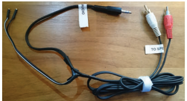
Figure 5. Hack an old audio cable to trigger the KA2284 board.
