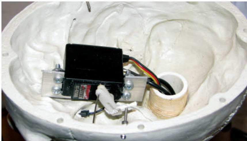
Figure 6. The servo is mounted inside the skull, and moves the jaw with a length of piano wire.
