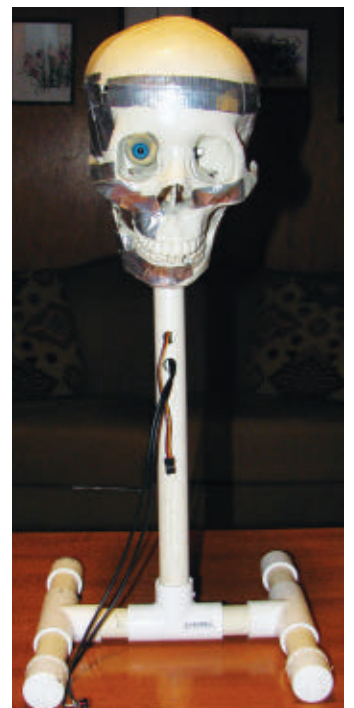
Figure 1. A PVC stand is needed to hold the skull due to its weight. One rubber eyeball is removed to show the LED in the back of the socket.
