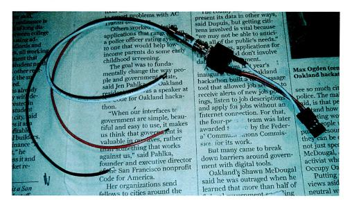
Use the multitester to confirm that white on one end connects to white on the other end, and the same for the other two colors. Also make sure there are no shorts between the colors. When you're satisfied it's all correct, put the plastic sleeve back onto the stereo plug.
