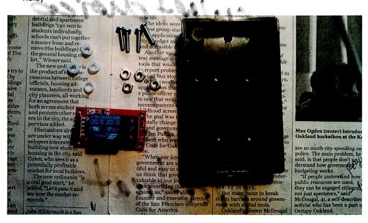
Put the screws into the holes on the relay board, and then thread the plastic tube sections onto the screws:
