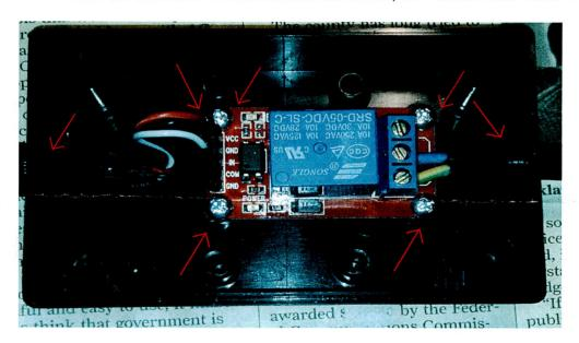
16. Screw the top on. Finally, put the top on and use the little bag of four screws to screw it closed.
