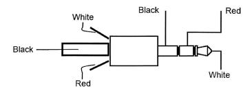
Test connections: Use the multitester to check for shorting between wires, and to check the wires connect to the right parts of the plug. Use pliers & crimp the wings on the black lug lightly around the wires.
