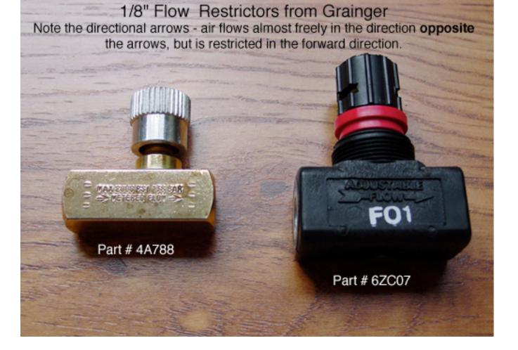
What are they used for? Making an animatronic move at the proper speed, for one thing. Pop-ups often reset as violently as they pop unless a flow restrictor is used on the exhaust cycle. Sometimes one is needed on the activation as well. Remember, violent action is what kills props ahead of their time, so here we have a means to avoid it. Grainger has them, as shown in the image above.
