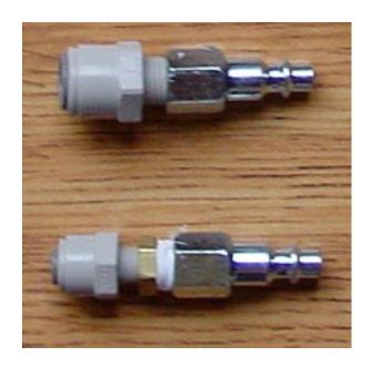
The plastic quick disconnect fittings work like this: you press down on the nylon ring around the tube and hold it, then pull out the tubing. It takes one or two tries to get the technique, but once it's mastered, quick disconnect air plumbing becomes much easier than wiring electricity.
