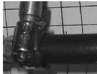
Push Hose Over Hose-Barb And use a Ring Clamp to tighten
