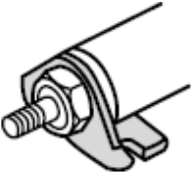
Nose Mounted cylinder using a Foot Bracket when cylinders need to stay locked in place
